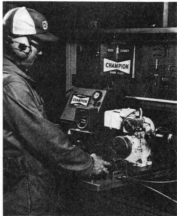
Figure 12-10. A small engine being tested on a dynamometer.
